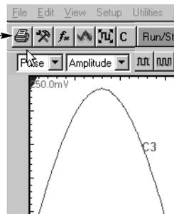
To copy a screen image into another application, choose the **Print to file** option in the print dialog. Save the screen image in a format that is compatible with your application, and then insert the screen image into your document.
