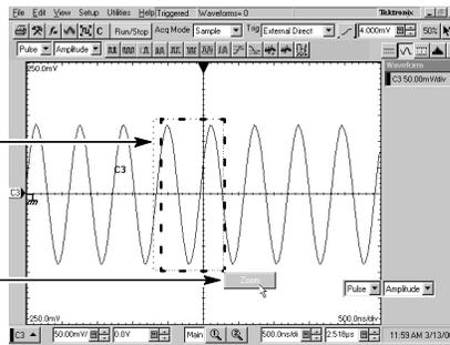
3 See the waveform reacquired with increased horizontal resolution.
