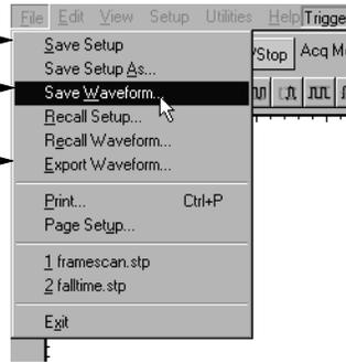
To export waveform data into a comma-separated ASCII file, click **Export Waveform** in the File menu.
